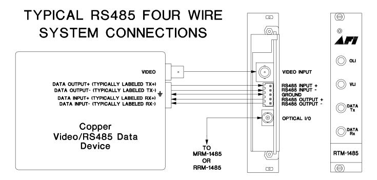
Also, please note that in four wire installations Data In on the RTM-1485-2F8 becomes Data Out on the MRM-1485-2F8 or RRM-1485-2F8 after going across the fiber. The reverse flow follows the same orientation.
