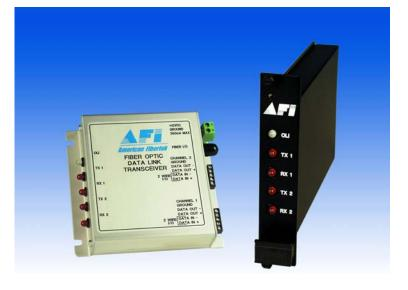
The American Fibertek 480 Series transmits and receives one simultaneous channel of data over multimode optical fibers. The system is comprised of two transceivers forming a point-to-point communications link. The system is designed to be completely transparent to data protocol and can be configured as RS-485 (2 wire or 4 wire), RS-422, RS-232 or Manchester Code. For ease of installation, diagnostic indicators provide a quick visual indication of system status.
