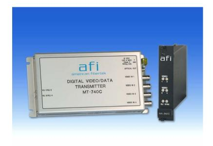
The American Fibertek 740C Series transmits four channels of high-quality digitized video on one multimode optical fiber. Designed to be completely transparent to all camera and monitor manufacturers, this system requires no field adjustments at installation or additional maintenance thereafter. Diagnostic indicators provide a quick visual indication of system status. The "Afinety" intelligent remote monitoring system is available on this product, please consult factory.
