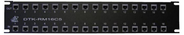
Power outages, surges, and voltage transients on data lines can be deadly to network equipment. DITEK's DTK-RM16C5 rack mount surge protector features individually replaceable surge protection modules for each data channel. The 16-channel DTK-RM16C5 will pass Gigabit Ethernet data without signal degradation.
