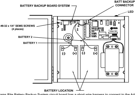
The Adams Rite Battery Backup System circuit board has a short wire harness to connect to the Adams Rite Power Supply circuit board. Install the orange connector of this harness into the BATT BACKUP connector of the Adams Rite Power Supply circuit board.
