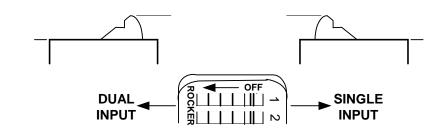
Two operating modes are available. Set the mode with switch 1 on dip switch SW1.
