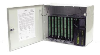
The PRO32IN interfaces with the intelligent control module (PRO32IC) providing 16 supervised alarm inputs and a dedicated power fail and panel tamper when tile mounted. An analog to digital converter samples the input values and the digitized result is filtered and processed. Filter parameters are configurable for each input point, resulting in the ability to specify a custom End-Of-Line (EOL) resistance value, sensitivity range and timing parameter.
