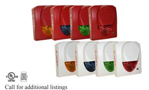
The CSH-1224W Strobe/Horn Series provides a wide range of candela light output options in a single device. The candela settings include a 12 or 24 volt DC operation for the 1-3 settings candela settings and 24 volt DC operation for the 1-6 candela settings. The candela setting is displayed through the front window and is selectable using a drum wheel.
