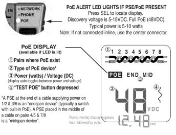
NOTE ON POWER (WATT) DISPLAY: To measure a device's power draw, the Power Panel must be connected inline (in between) the PSE switch and the PoE device.
