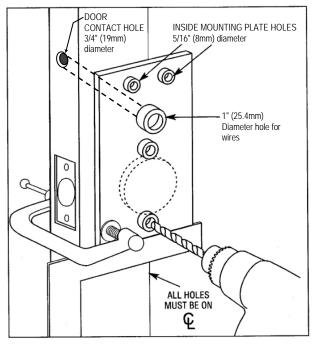
FIG. 2: ALARM LOCK INSTALLATION JIG
