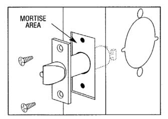
FIG. 3: LATCH INSTALLATION
