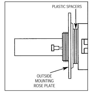
FIG. 9: ADJUST DOOR THICKNESS
