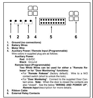
FIG. 24: WIRE CONNECTIONS
