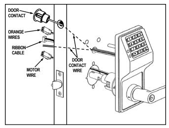
FIG. 7: INSTALL OUTSIDE LOCK BODY
