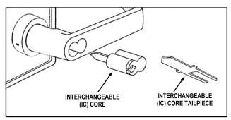
FIG. 22: INSTALL INTERCHANGEABLE (IC) CORE
