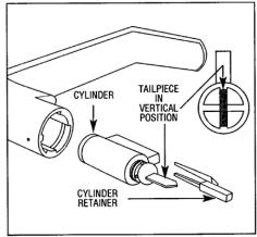
FIG. 20: STANDARD CYLINDER-LEVER, TAILPIECE AND RETAINER.
