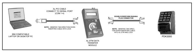
Scenario 2 Create the program in DL-Windows and transfer the program from your computer to an AL-DTM (via an AL-PCI cable)... then transfer the program from the AL-DTM to the lock(s) (via a double-ended mini banana plug). The hand-held AL-DTM is useful because you do not have to transport (or find electricity for) your computer. Data can also flow in reverse, from the lock, through the AL-DTM, back to the computer for examination.
