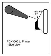
Infrared LED Infrared Reader Place Infrared Reader (on printer) in front of the Infrared LED (on lock)
