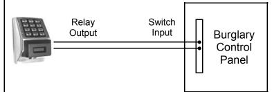
Alarm Panel with Switched Input for Disarming
