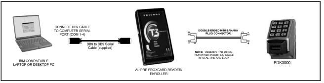
Scenario 3 Enroll ProxCards® quickly into DL-Windows, then transfer this new ProxCard® data from the computer through the AL-PRE to the lock (thus avoiding the need to use an AL-PCI cable). For PDK series locks only.
