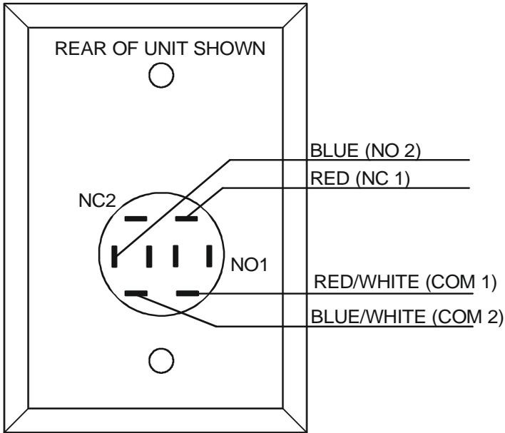
THE TWO TERMINALS IN THE CENTER OF THE SWITCH ARE FOR OPERATION OF AN LED ILLUMINATOR FOR THE SWITCH. THIS ILLUMINATOR IS FURNISHED ON SECURITRON'S PB3 SERIES. THE PB3E SERIES DOES NOT INCLUDE ILLUMINATION.
