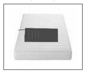
Mount Sensor Pad <u>ACROSS</u> Bed with wire leads routed toward back to sensor unit.
