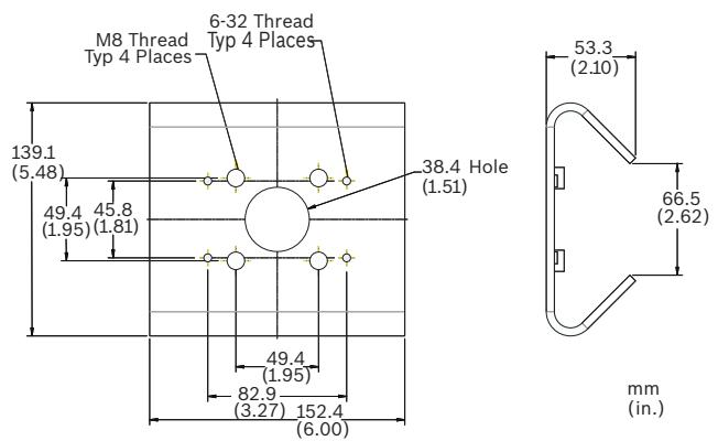
**VDA-PMT-DOME –Pendant Pipe Mount**
