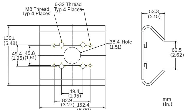
**VDA-PMT-DOME –Pendant Pipe Mount**
