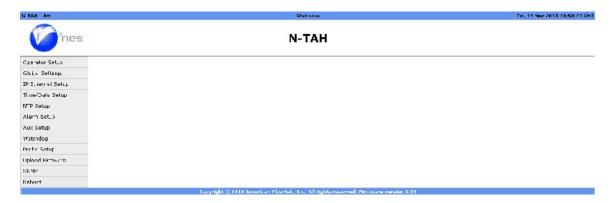
The N-TAH web interface screens use a common design in which the screen is divided into three sections. Across the top of the screen is a title bar which contains the user-settable device name and device location strings, and the current time and date setting.
