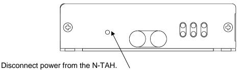
With a paperclip or other small object, press and hold the reset button.
