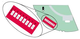
You can find the Address Switch Settings using the chart on page 3, or by calculating the decimal number of the address.
