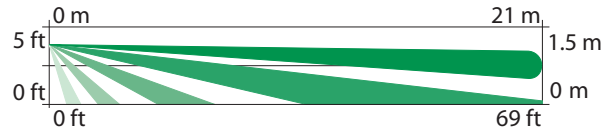
Side View Optional Long Range Coverage: 21 m x 3 m (70 ft x 10 ft)
