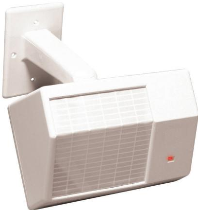
The MX794i is a PIR intrusion detector that provides a variety of coverage patterns through the use of interchangeable mirror modules. It is designed to connect to the Multiplex Bus of a control panel and optionally to an auxiliary 12 VDC power source. It is compatible with DS7400, DS7400X, or DS7400Xi Series Control Panels, with a DS7430 or DS7436 Multiplex Expansion Module, or with GV2 and G Series Control Panels with a D8125MUX Module installed.
