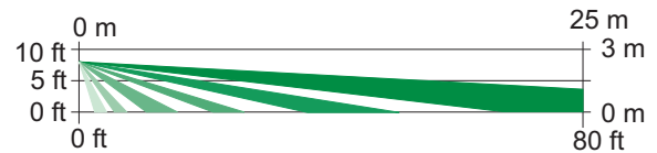
Side View Optional Barrier Coverage: 15 m to 25 m x 5 m (50 ft to 80 ft x 16 ft)
