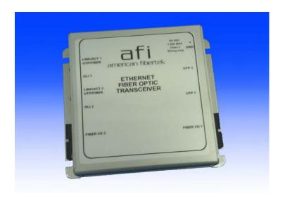
The American Fibertek 49SL-PoE+ Series transmits and receives (2) copper 10/100/1000 Base-T Ethernet signals at the RJ45 ports and (2) optical 1000 Base-X over 1 or 2 singlemode fibers. The system is comprised of two or more units forming a communications link.
