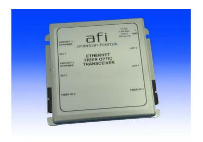
The American Fibertek 49 Series transmits and receives (2) copper 10/100/1000 BaseT Ethernet signals at the RJ45 ports and (2) optical 1000 Base-X over 1 or 2 multimode fibers. The system is comprised of two or more units forming a communications link.
