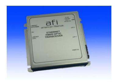
The American Fibertek 46-PoE Series transmits and receives (2) copper 10/100 Base-T Ethernet signals at the RJ45 ports and (1) optical 100 Base-FX over 1 or 2 multimode fibers. The system is comprised of two units forming a point-to-point communications link.
