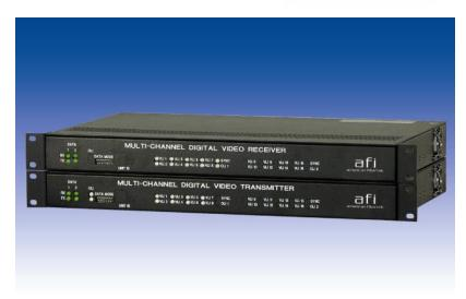
The American Fibertek 985C-SL Series transmits 8 channels of high-quality 10 Bit digitized video and two channels of user selectable multi-protocol data on one singlemode optical fiber using WDM technology. The available data channels are RS485 (2 or 4 wire), RS422, RS232 and Manchester. Data rates up to 115 kbs are supported.
