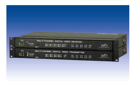
The American Fibertek 985C Series transmits 8 channels of high-quality digitized video and two channels of user selectable multiprotocol data on one multimode optical fiber using WDM technology. The available data channels are RS485 (2 or 4 wire), RS422, RS232 and Manchester. Data rates up to 115 kbs are supported.
