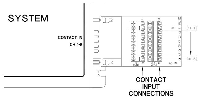
Contact closure input connections are made via terminal blocks attached to the right side of the unit. Please note that the two Channel 1 inputs begin at the second terminal screw closest to the fiber connection on each of the two nine pin terminal strips. Channels 2 through 8 connections continue down the terminal strip. For optimum performance the copper cables carrying the contact closure signal should be the shortest length of wire practical.
