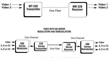
A = AUDIO D = DATA CC = CONTACT CLOSURE MODULATORS AND DEMODULATORS
