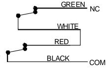
SERIES CONNECTION OF SWITCH AND TAMPER NC LOOPS TO MAINTAIN BOTH FEATURES WITH A SINGLE ALARM POINT.
