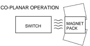
TO ENHANCE DEFEAT RESISTANCE, THE MAGNET PACK CAN ONLY BE READ IN A NARROW ANGLE IN FRONT OF THE SWITCH.
