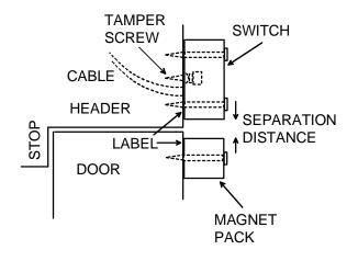
shown. Drill 7/64" (2.75MM) diameter pilot holes for the #8 mounting screws.
