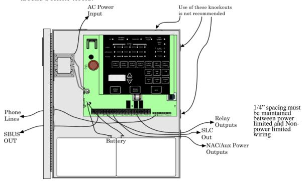
Figure 3-1 Wire Routing Example
