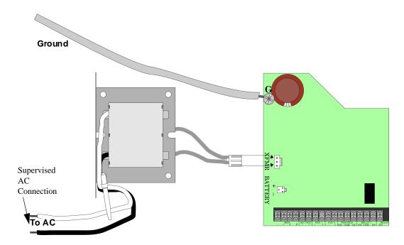
Figure 4-2 120/230 VAC Power Connection
