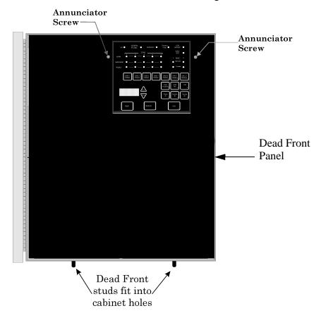
Figure 4-1 Dead Front Installation and Removal
