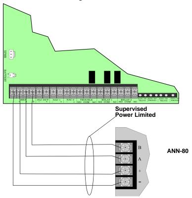
Figure 4-5 SBUS Class B Wiring
