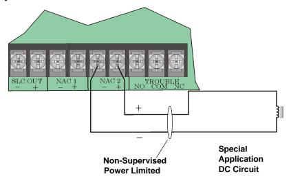
Figure 4-12 Example of an Auxiliary Power For Door Holder
