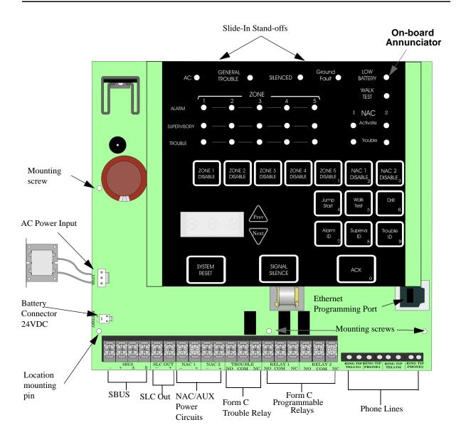
Figure 3-2 Model MS-25 Assembly
