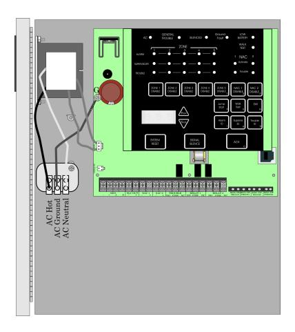
Figure 4-3 AC terminal Block Connections
