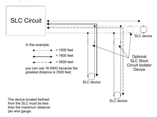
SLC device max loop resistance = 40 ohms
