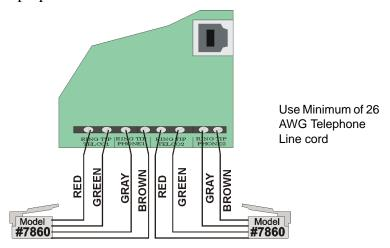
Figure 4-10 Connection of Telephone Lines
