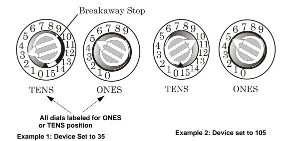
Figure 5-4 SLC Device Addressing Using Rotary Dials
