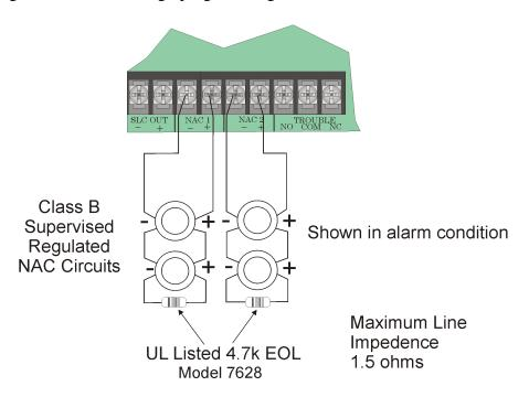
Figure 4-11 Class B Notification Appliance Circuit Wiring
