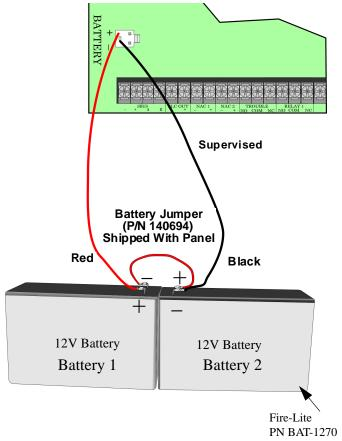
Figure 4-4 Battery Connection
