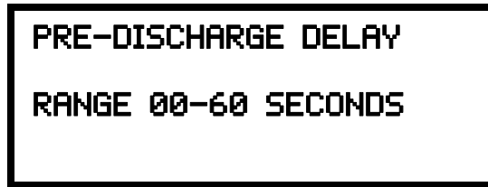
Pre-Discharge Setup Screen
