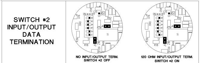
To open the MRM-61, remove the screw on the bottom of the module. Also remove two screws holding the end panel to the chassis on the side with the video and data connections. Slide PCB assembly out of chassis to access the switch and jumper locations.
