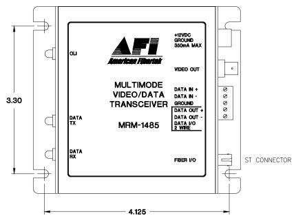
Data input and output connections are made via a terminal block on the right side of the unit. Follow label on unit for proper orientation of RS485 data input and output. Please note that two wire applications utilize the four wire data out + and data out - terminals.
