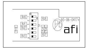
Please remember when using offset bias switches that they must be used in pairs. If switch # 1 is up then switch # 3 must also be up. The same situation applies for switch # 4 and switch # 6. Also, if using offset bias, it is important that the corresponding termination resistor switch be in the on (up) position. Using offset bias without a termination on the line will cause communications to fail. An explanation follows on general bias and termination guidelines.
