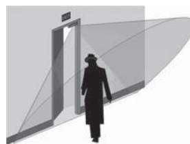
Embedded CCTV captures full facial view of persons exiting door
