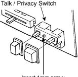
Insert 1mm screw in hole to hold open.
