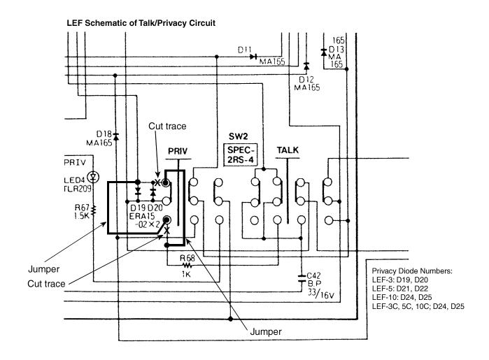
Solder two jumpers in place as shown above. Cut traces where marked with an "X".
