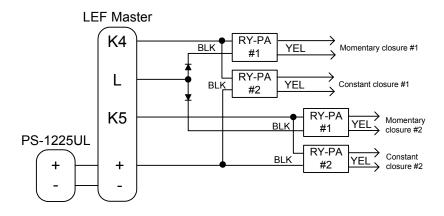
Each station that requires both a constant closure and momentary closure when a channel is selected requires the following: 2 RY-PA relays 2 Diodes (1N4001)
