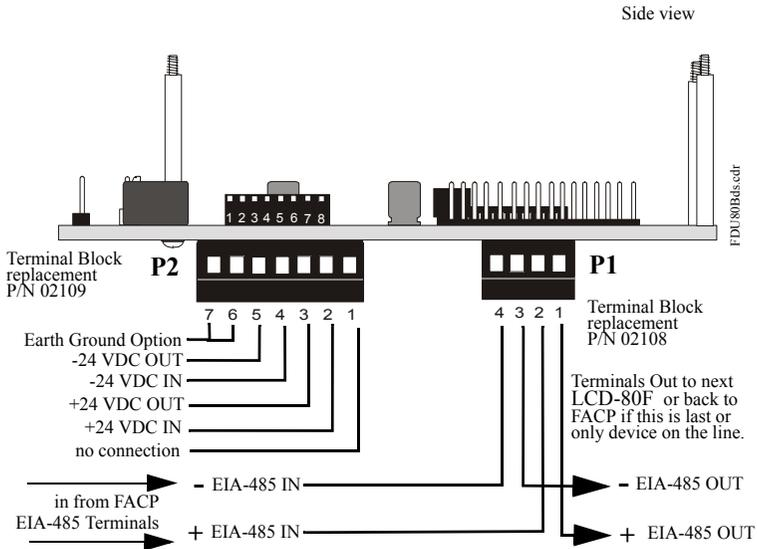
*Note: These connections must be power-limited and the +24 VDC nominal power input must be filtered and nonresettable.*
