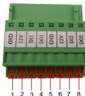
To connect input devices (DI), map the pins to one of the pin combinations below:
