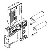
REMOVE the batteries, UNPLUG the cable carefully, and SEPARATE the lock and reader to prepare for installation.
