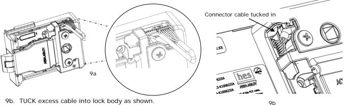
9b. TUCK excess cable into lock body as shown.
