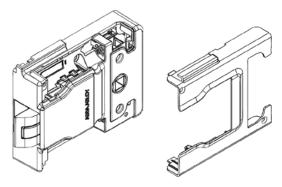
CONNECT the wire (the wire is keyed) from the reader to the socket in the lock battery
