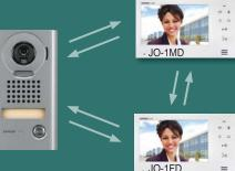
\* The JO Series **does not** support internal communication. The JO-1MD and the JO-1FD can only converse together when they are both in active communication with the door station.
