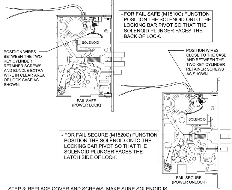
STEP 3: REPLACE COVER AND SCREWS. MAKE SURE SOLENOID IS PROPERLY POSITIONED IN COVER SLOT.
