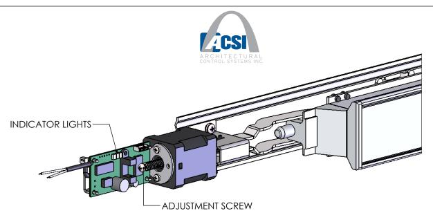
**Motor Drive Electric Latch Retraction Adjustment:**
