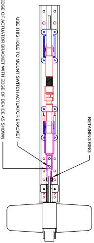
LINE UP EDGE OF ACTUATOR BRACKET WITH EDGE OF DEVICE AS SHOWN
