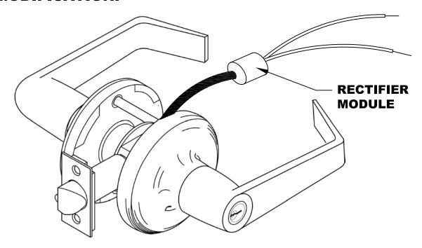
TERMINATE THE TWO BLUE WIRES FROM LOCK TO THE ELECTRIC POWER TRANSFER DEVICE USING 22 AWG WIRE. USE PROPER CRIMP SPLICES OR WIRE NUTS FOR TERMINATING CONNECTIONS. (NO POLARITY OF WIRES IS REQUIRED)
