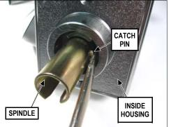
Press the catch pin as shown, then pull the inside housing off spindle.
