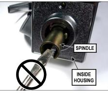
Do NOT insert a screwdriver or other tool into the spindle to release the catch pin, as the catch spring is easily damaged.
