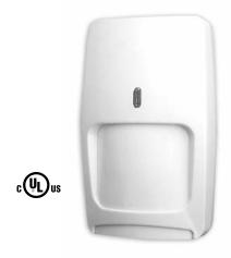
The DT7235T DUAL TEC® Motion Sensor provides reliable protection with pet immunity for up to 100 lbs. in a simple installation configuration that requires no adjustments. Optimum performance is achieved using K-Band microwave technology and Uniform Sensitivity Optics.
