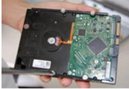
Figure B-14 Loosening the Four Screws in the HDD Housing
