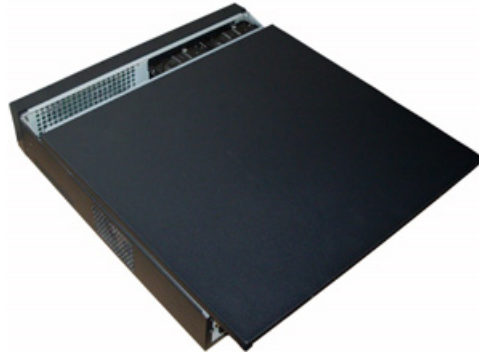
Figure B-17 Replacing the NVR Cover
