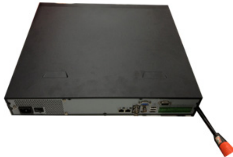
Figure B-8 Removing the NVR Cover
