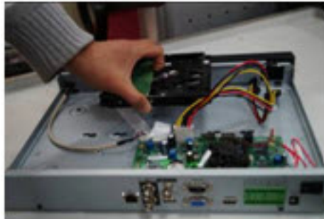
Figure B-3 Placing the HDD
