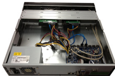
Figure B-16 Connecting the HDD and the Power Cable
