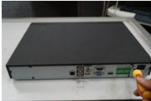
Figure B-7 Securing the NVR Cover
