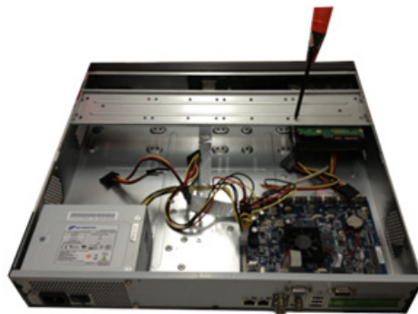
Figure B-10 Placing the HDD
