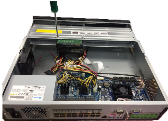
Figure B-15 Placing the HDD
