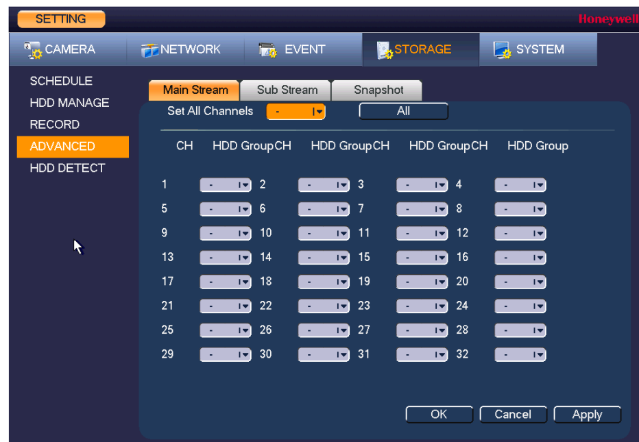
Figure 9-4 Main Stream Storage Configuration Tab
