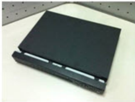
Figure B-6 Replacing the NVR Cover
