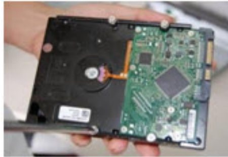
Figure B-9 Loosening the Four Screws in the HDD Housing
