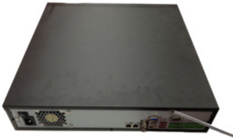
Figure B-13 Removing the NVR Cover
