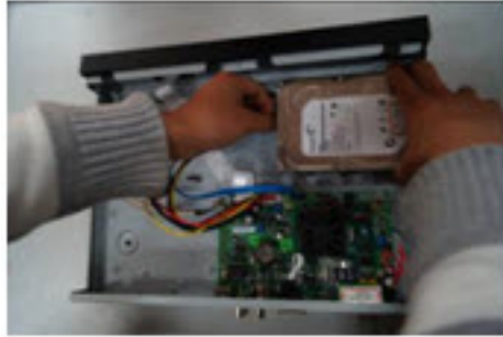
Figure B-5 Connecting the HDD and the Power Cable
