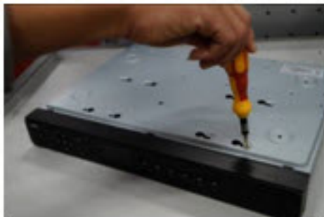
Figure B-4 Securing the HDD to the NVR Housing
