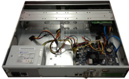
Figure B-11 Connecting the HDD and the Power Cable
