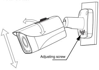
2. Adjust the bullet camera to the desired field-of-view angle, and then re-tighten the adjusting screw to secure the camera in place.
