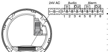
c. Connect a twisted pair (UTP) cable from each peripheral alarm contact to each alarm input on the terminal block. For detailed audio and alarm configuration information, refer to the appropriate user guide located on your software DVD.
