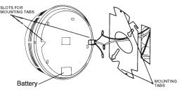
3. Place the heat alarm up to the mounting plate, rotating it clockwise until alarm firmly snap locks into place. Keep the heat alarm parallel to the mounting plate so upper and lower tabs on the plate seat correctly into the heat alarm.
