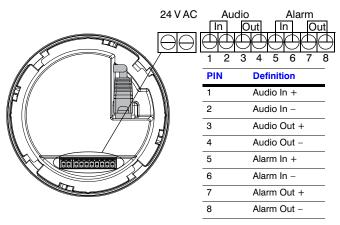
Connect a twisted pair (UTP) cable from each peripheral alarm contact to each alarm input on the terminal block. For detailed audio and alarm configuration information, refer to the appropriate user guide located on your software DVD.
